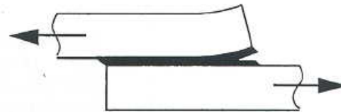
d. Cohesive Failure (Peel)
