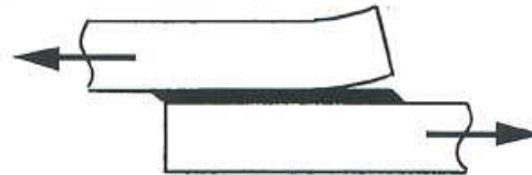
f. Adhesive Failure (Peel)
