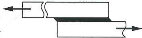
a. Adherend Failure (Outside of Joint)
